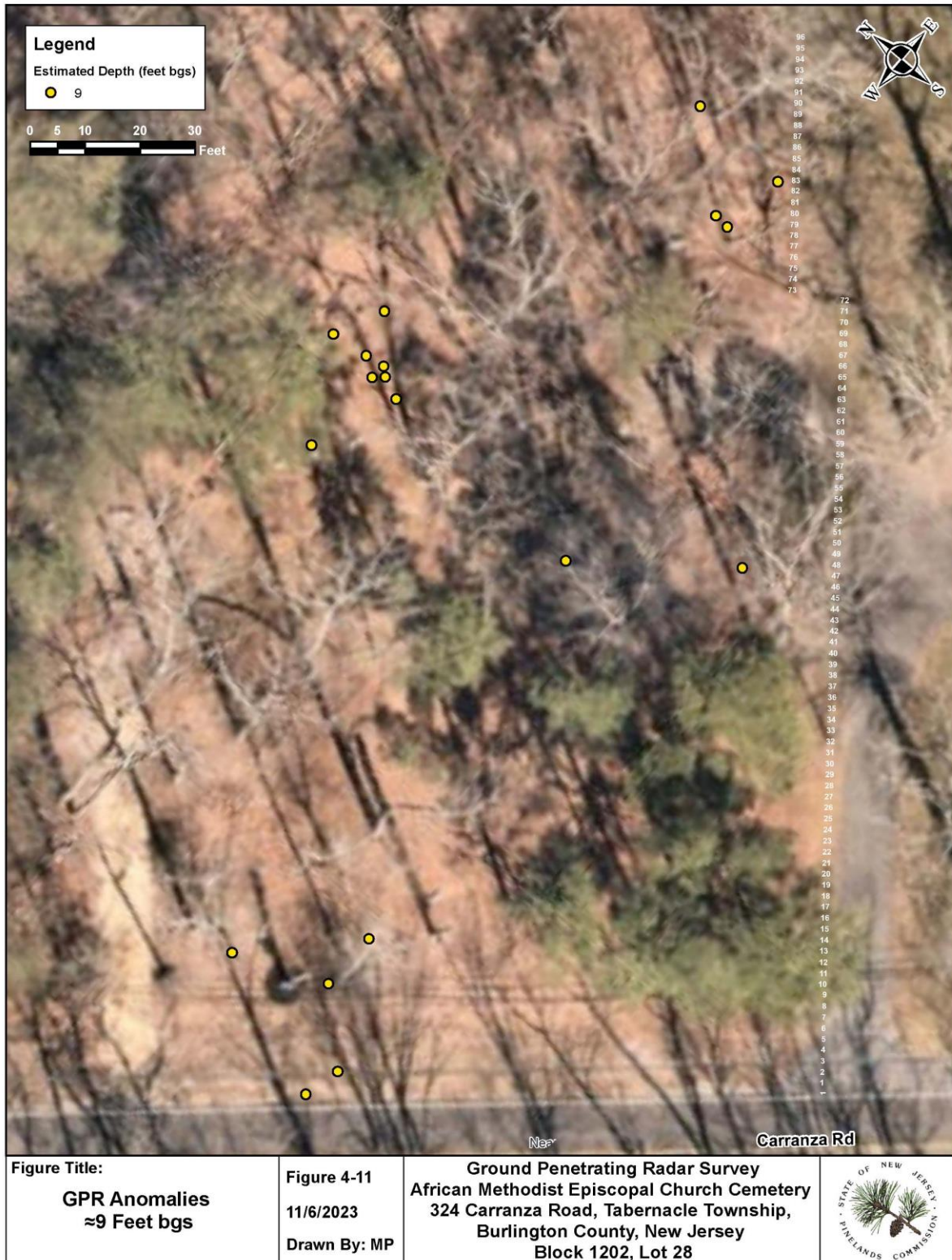
Figure 4-11: Depth of Anomalies approximately 9 feet below ground surface
