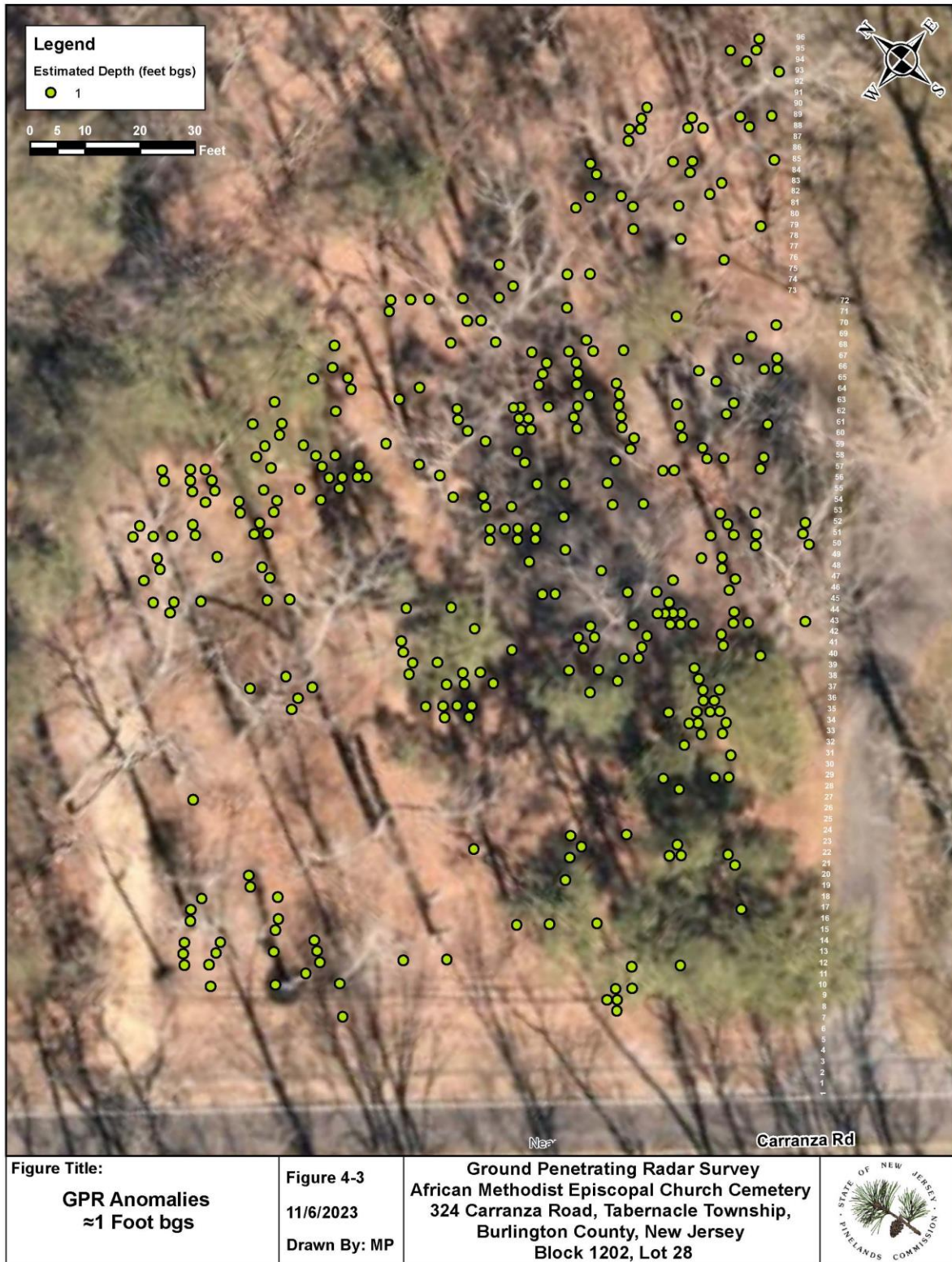
Figure 4-3: Depth of Anomalies approximately 1 foot below ground surface
