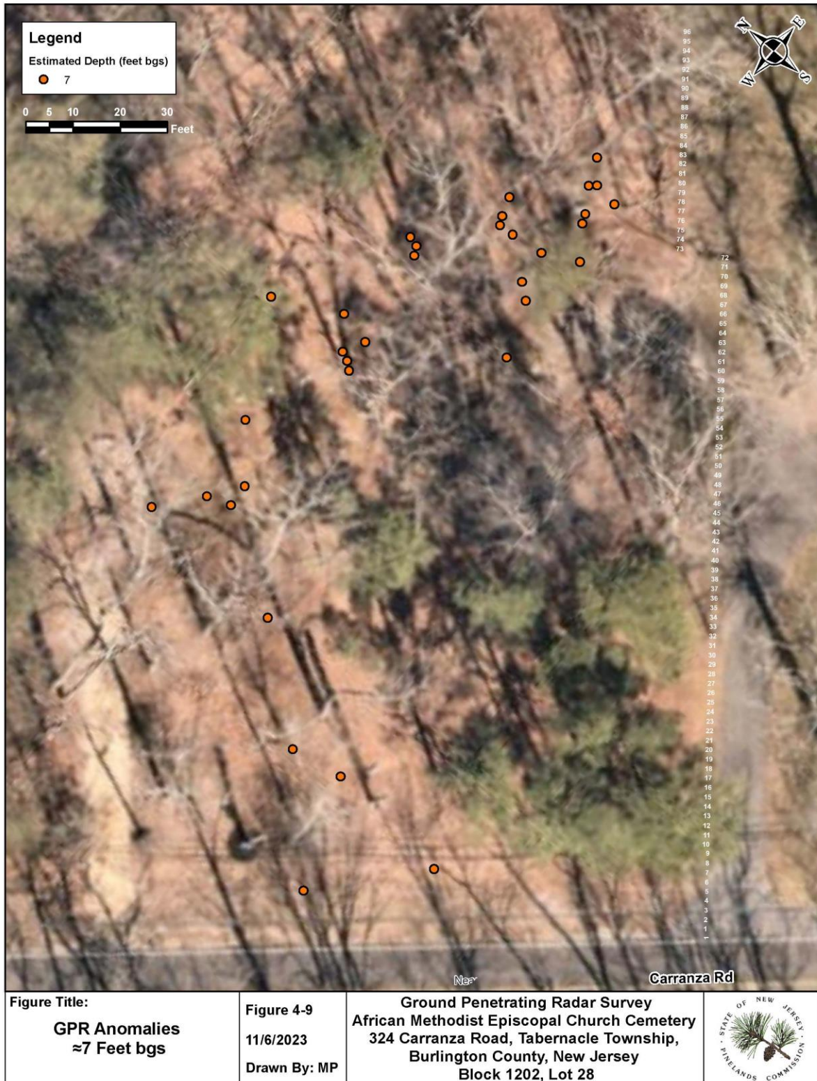
Figure 4-9: Depth of Anomalies approximately 7 feet below ground surface
