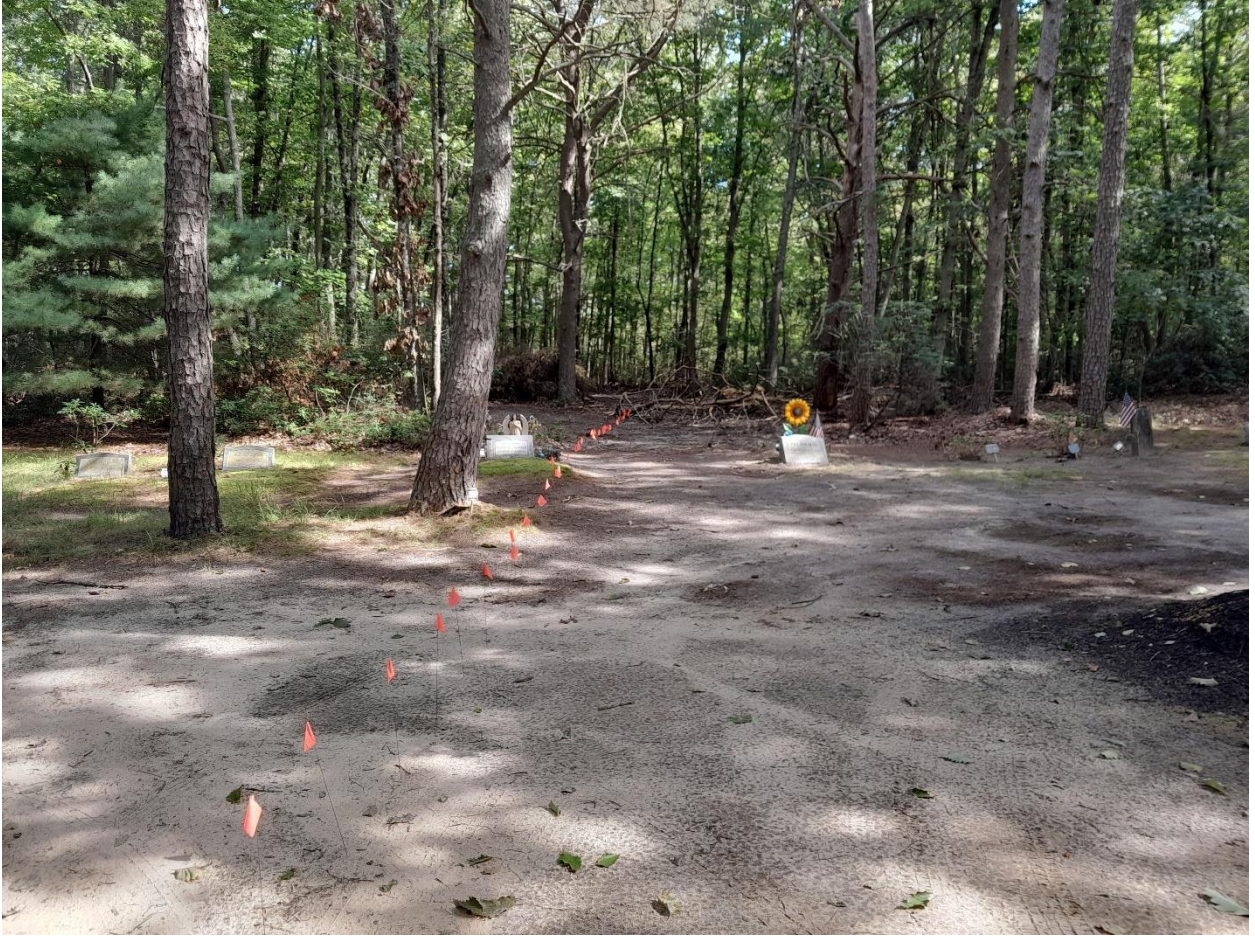
Plate 4-1: Flagging pins marking baseline of GPR transects. View to the northeast.
