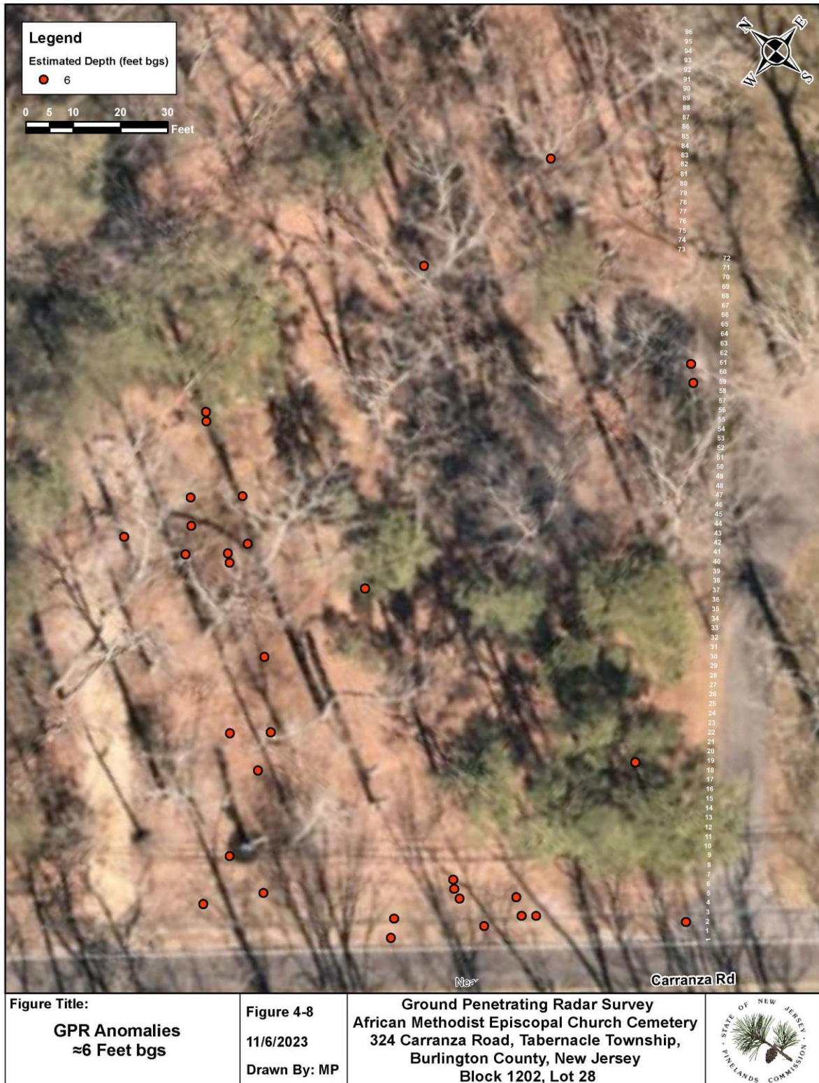
Figure 4-8: Depth of Anomalies approximately 6 feet below ground surface
