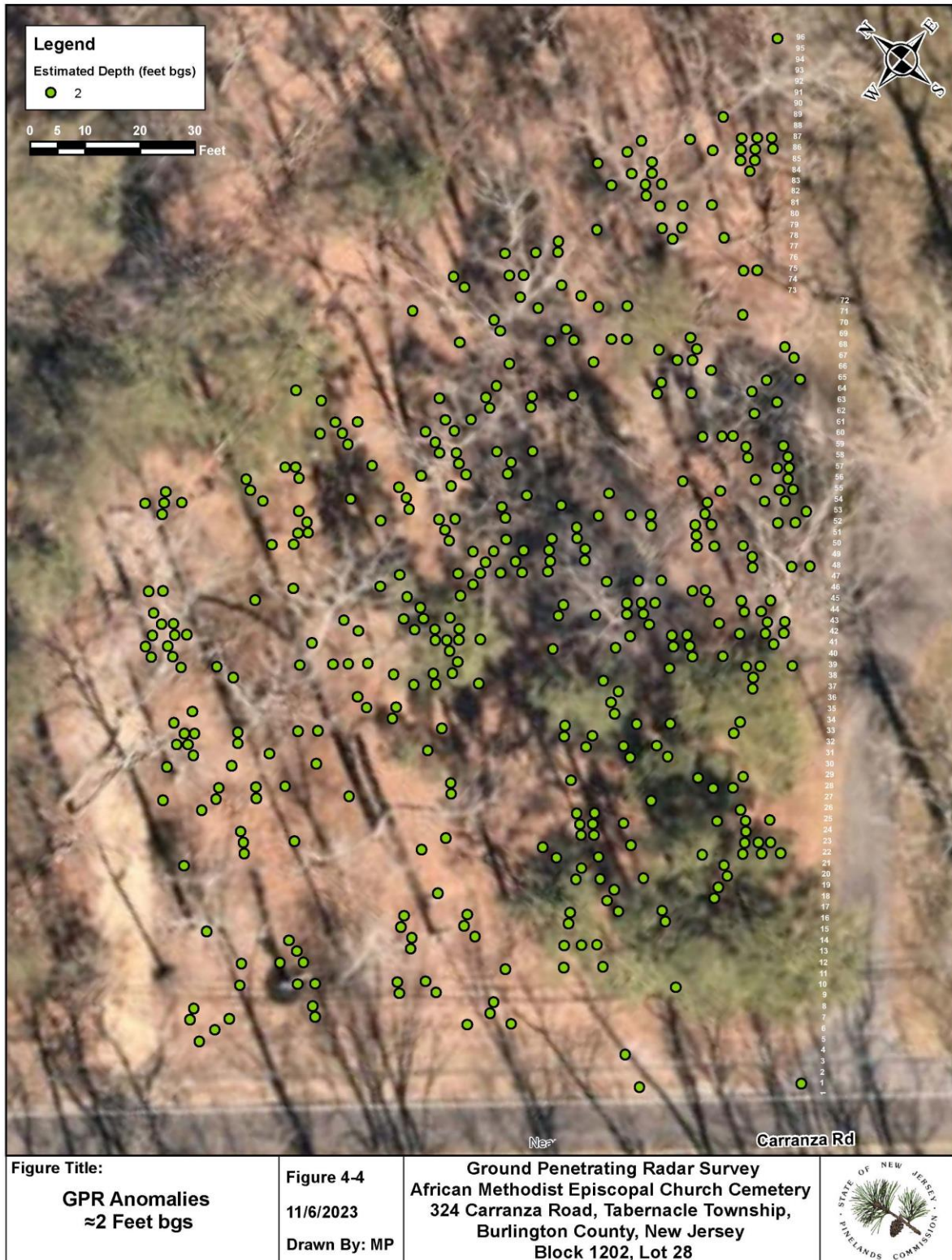
Figure 4-4: Depth of Anomalies approximately 2 feet below ground surface
