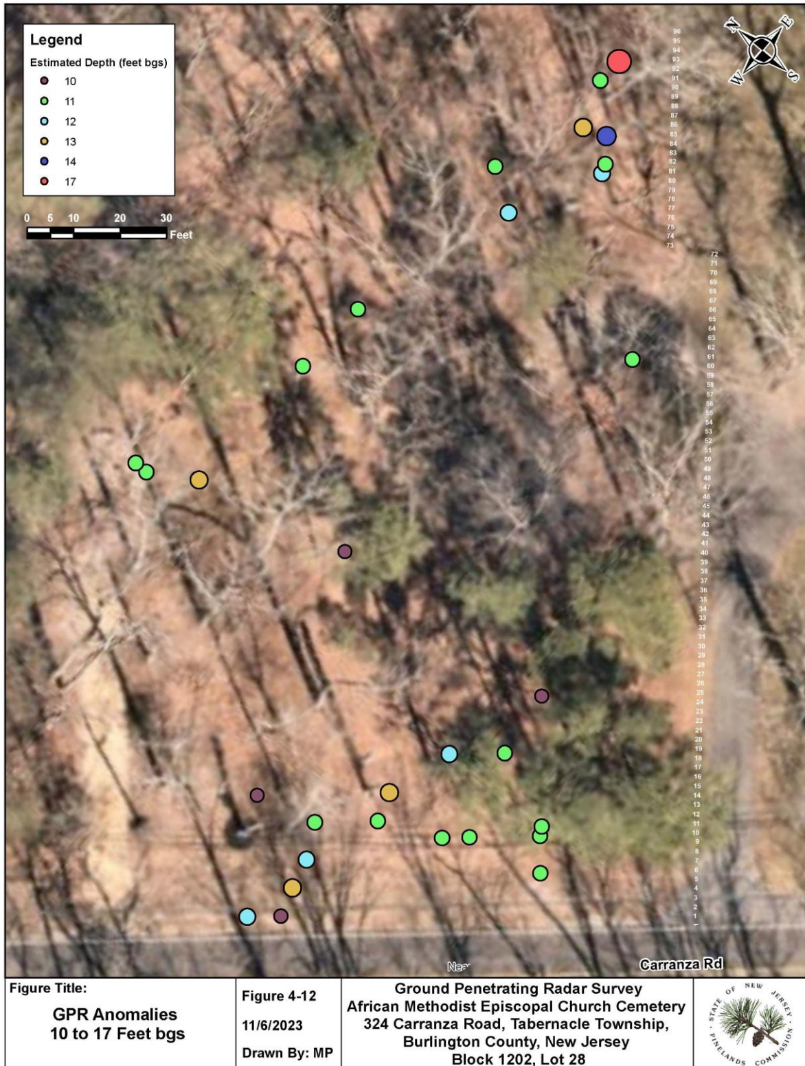
Figure 4-12: Depth of Anomalies between 10 and 17 feet below ground surface
